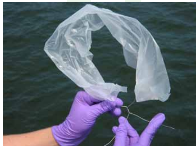
Above: The sampling film prepared and tied to a wire.
